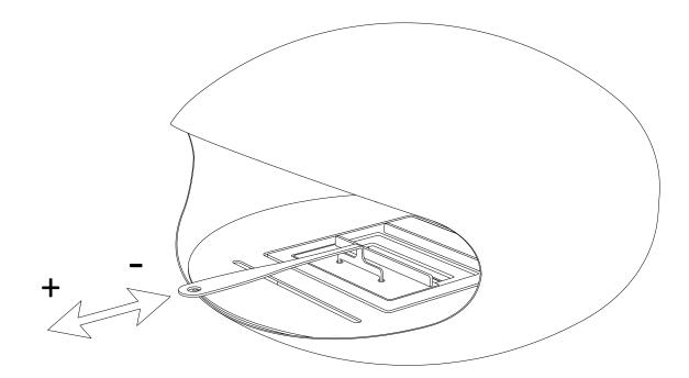
To regulate the flame, insert the tips of the *Sliding Lid Handle* into the holes of the *Sliding Lid* of the *Combustion Chamber* and slide backwards or forwards to regulate the flame size.
