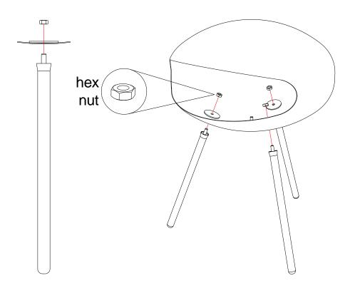
Screw the three Legs from the bottom of the Main Body and secure Legs from the inside of the Main Body with the three hex nuts.
