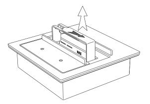
When the flat ends of the Lifting Handles are all the way inside the Combustion Chamber, slide the handle into the open position as far as it will go. Grip the handles Parts A and Part B firmly with one hand in the fully open position, then lift and insert the Combustion Chamber inside the Mount Plate.
