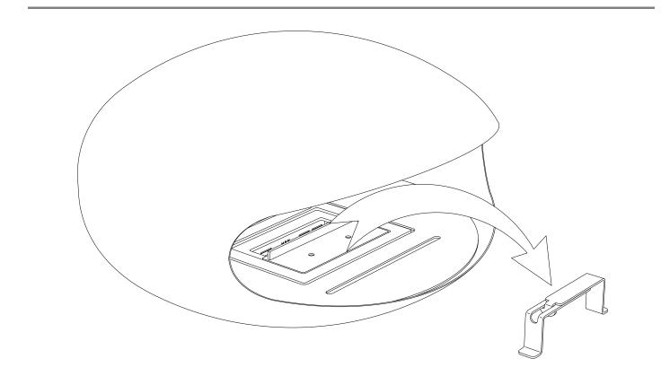
Your Cocoon Burner is now ready to use, follow the steps on the following pages to correctly and safely fill, ignite, adjust, shut off and refill the Combustion Chamber. Always make sure the Lifting Handles are removed from the Combustion Chamber as shown above when it is not in use otherwise these parts will become too hot to touch and may cause injury.
