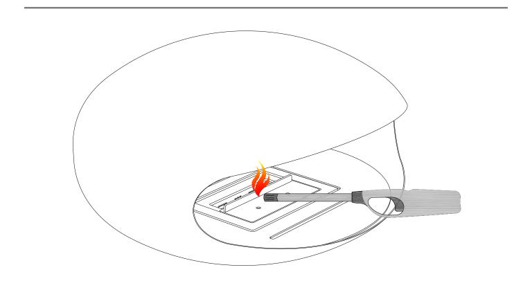
Using a long arm fire lighter and standing at a safe distance from the Combustion Chamber carefully introduce a flame as indicated above to ignite the Combustion Chamber. Always make sure there is a Class B fire extinguisher close at hand when igniting the Combustion Chamber.
