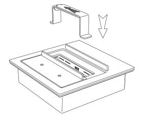
With the handle in the closed position, lower the flat tabs at the bottom of the Lifting Handle into the Burner Vent opening of the Combustion Chamber.
