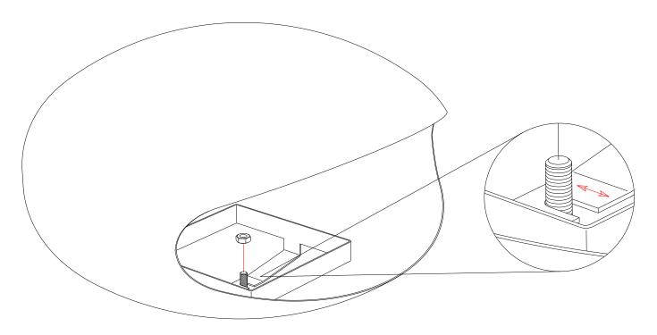
With the Removable Tray Bracket and hex type nut loosely in place, adjust the Removable Tray Bracket backwards or forwards so that the front edge of the Mount Plate (A) sits just below the front bottom lip of the opening in the Main Body (B). Once this adjustment is done, then tighten the hex type nut to secure the Removable Tray Bracket in place.
