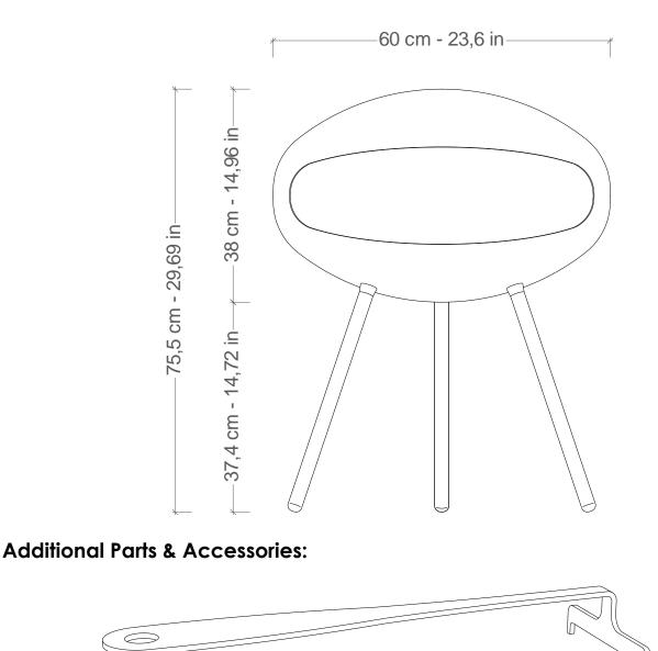
The **Sliding Lid Handle** is used to adjust the intensity of the flame by sliding the *Sliding Lid* backwards and forwards, and also to extinguish the flame by sliding the *Sliding Lid* into the closed position.
