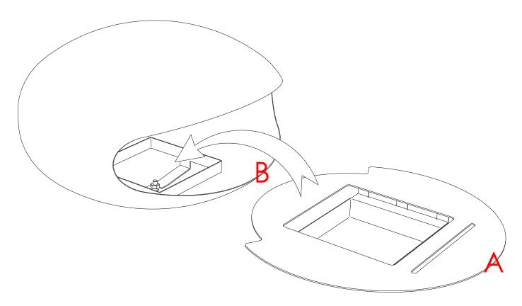
NOTE: adjustment instructions on the following page showing relative positions of (A) and (B) shown above are critical to the airflow inside the *Main Body* and therefore critical to the proper functioning of the *Combustion Chamber*.
