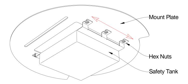
Further adjustment to the position of the Mount Plate can be achieved by loosening the 6 hex nuts below the Mount Plate and sliding the Safety Tank front to back slightly. Always make sure that the Safety Tank below the Mount Plate is properly secured after this adjustment.
