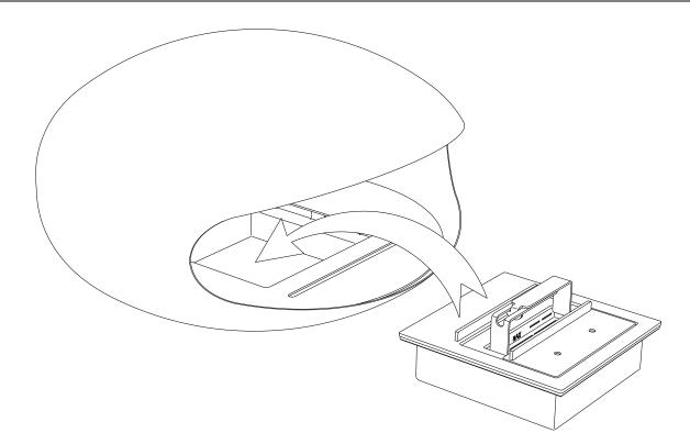
With the Mount Plate in the correct position and secured in place with the hex nut, the Combustion Chamber can now be placed inside and taken off the Mount Plate opening using the Lifting Handles supplied as shown on the previous pages.
