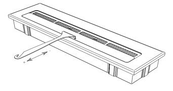
The flame intensity is adjusted by inserting the *Sliding Lid Handle's* tip into the corresponding holes in the *Top Plate Sliding Lid* as indicated above. Note the flame intensity takes a few minutes to change after an adjustment has been made.
