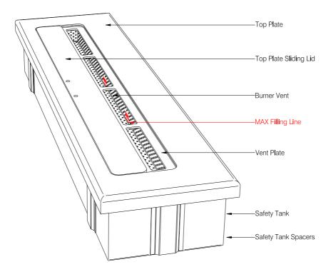
Fill the Linear Burner Fuel Tank to the Fill Line until the fuel becomes visible at the bottom of the Burner Vent. Fill using the Fuel Pump supplied or a funnel.
