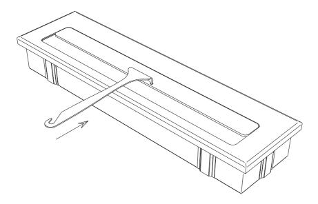
Using the *Sliding Lid Handle*, pull the *Sliding Lid* to the front / closed position. Should the flame not extinguish with the first try please repeat until extinguished. It should be a swift action coupled with downward pressure.
